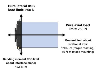
Figure 16: Robotic arm load limits for preliminary design.
