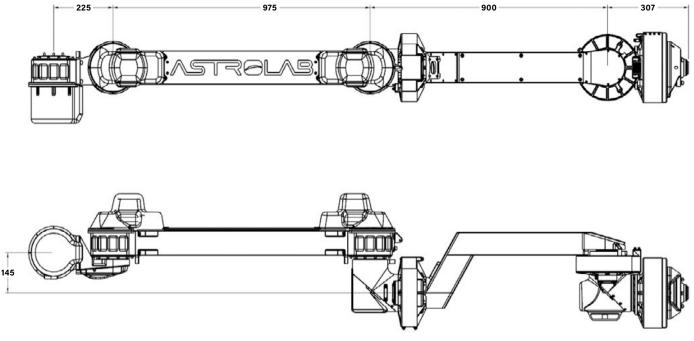
Figure 6: FLEX robotic arm dimensional layout.
