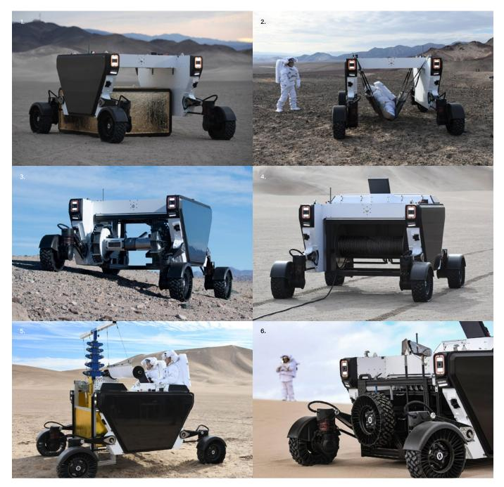
Figure 4: FLEX's innovative wheel-on-limb system allows the rover to retrieve, transport, and deploy payloads that conform to common interface standards. Examples include: 1. Outpost Logistics; 2. Crew Rescue 3. Marsupial Rover, 4. Cable Spool, 5. Vertical Solar Array Tower, 6. Crew EVA Equipment.
