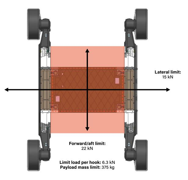
Figure 15: Underslung payload interface design limits.
