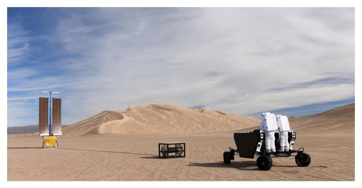
Figure 12: Field test deployment of a vertical solar array tower (a top-deck payload) and cable spool (an underslung payload). The rover's removeable crew interface is another example of a top-deck payload.
