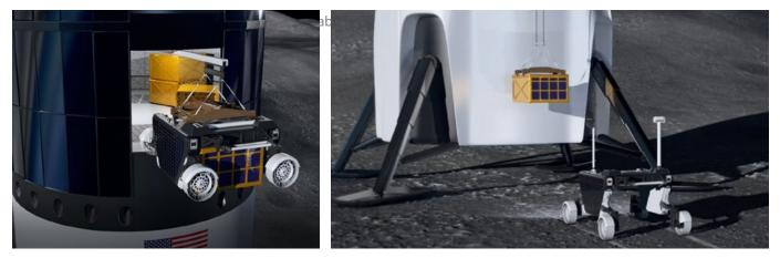
Figure 2: The Astrolab intermodal payload standard provides the ability for a single lander to deliver many payloads that a FLEX rover can transport.
