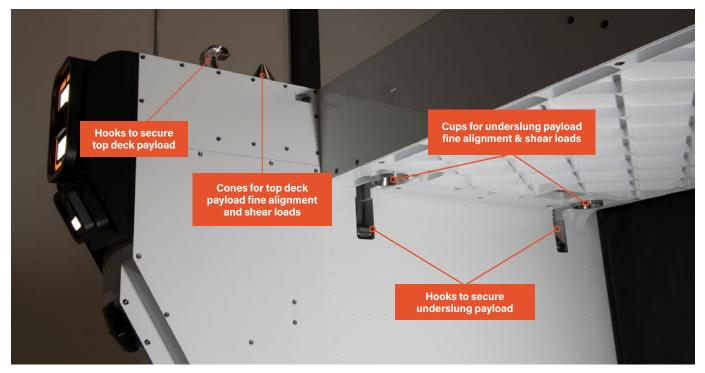
Figure 7: FLEX has two top-deck payload interfaces and one underslung payload interface.
