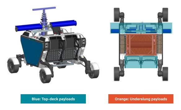
Figure 11: Example Terrestrial prototype configuration: Crew deck and vertical solar array tower top-deck payloads with 1.0 m standard-size underslung cargo.
