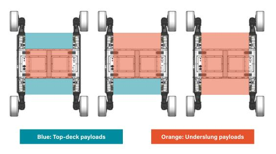
Figure 8: Top-view illustration of select FLEX payload configurations.
